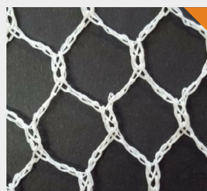
Hexagonal warp knitted net
